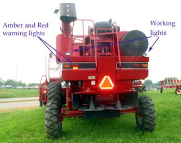
Photo 3: This combine shows a good SMV, amber and red retroreflective tape, and red and amber lights. Not visible are headlights. The working lights should not be used when travelling on public roadways.
