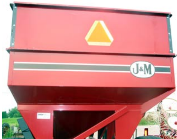
Photo 2: When illuminated with low beam headlights SMV emblems should be seen as a hollow bright red triangle. At night the triangle should be visible at 600 feet.
