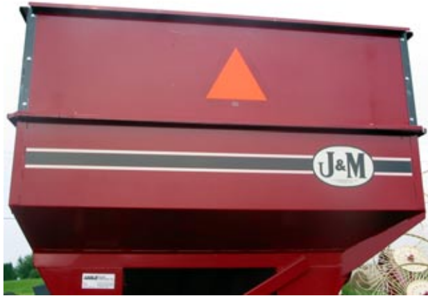
Photo 1: A properly placed SMV emblem that is clean, bright, and not obstructed. The red-orange fluorescent equilateral triangle should be the most obvious feature of the emblem.
