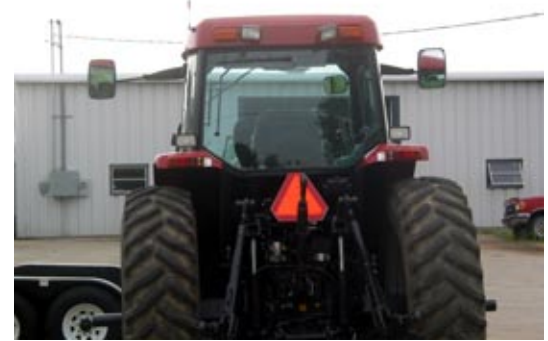
Photo 1: A properly placed SMV emblem that is clean, bright, and not obstructed. The red-orange fluorescent equilateral triangle should be the most obvious feature of the emblem.
